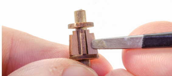
172. Slide part #77 onto the dowel and sit parts #78 into the slots as shown. You can also slide part #79 onto the dowel. The is the one shown at the top here. When all parts #78 are in place, slide down part #79 onto them and lock them into place.
