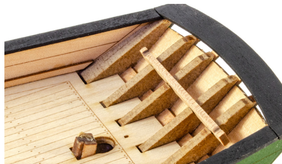
139. Glue into place across the notches on the stern timbers.
