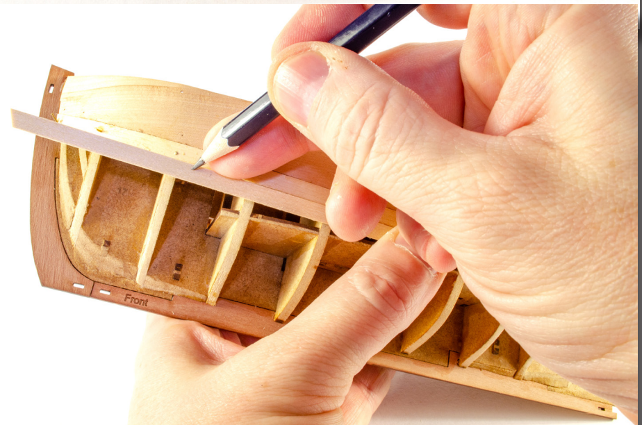
76. You will now need to taper the planks, or they simply won't lie flat on the bulkheads. While more knowledgeable and experienced modellers will have their own system of planking, this manual generally caters to those who are only starting the hobby. To taper a plank, run it underneath the previous one, and mark the point at which it tries to cross over the previous one.
