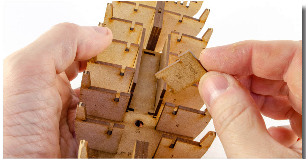
27. Now take part #24 (engraved as FRONT), and glue into position in the deck slots and against parts #22.
