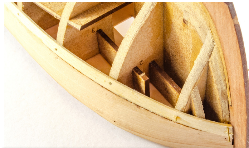
75. In this picture, you can see that the planks lie properly against the bulkheads, with no gaps. Add another plank to the opposite side of the hull.
