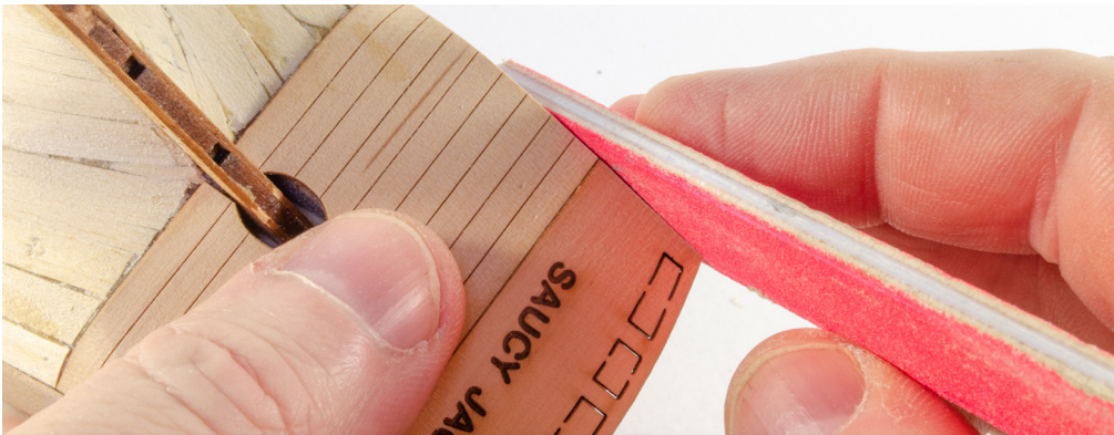
97. Now sand the rear sides of the hull so that the parts you just fitted are flush to the hull sides/planks/bulwarks.
