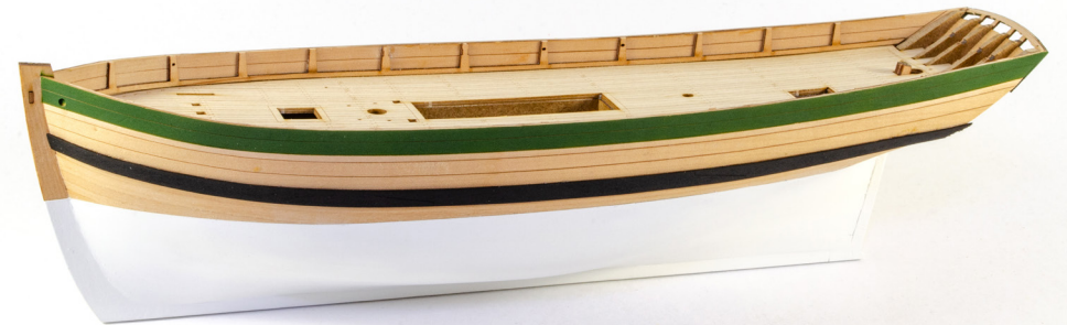
129. Paint those parts black and then fit to the hull. The upper edge of these parts will run along the lower engraved line on the bulwarks and hide the joint between the bulwark and planking. You may need to adjust the forward angle of the parts, and also bevel the inside front edge a little, so it sits against the prow properly. For fixing these, we use CA gel, applied in small spots. This gives the modeller some time to work their way along the part to fit it properly.
