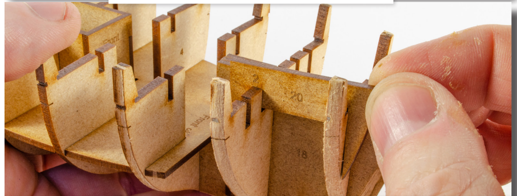
32. Slot (DO NOT GLUE) into position across the innermost slots on the top of bulkheads #1 and #2.
