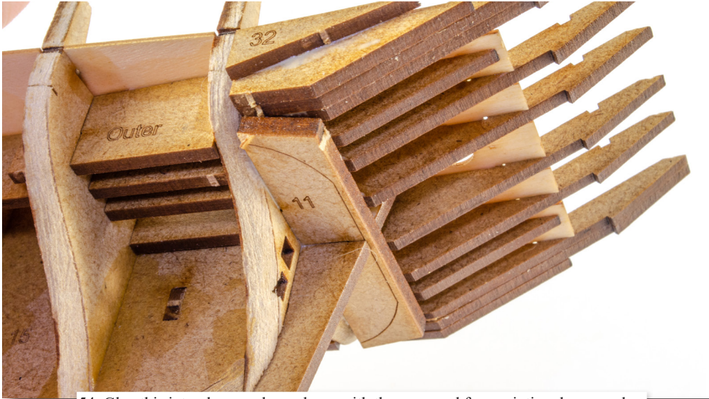
54. Glue this into place as shown here, with the engraved face pointing downwards.
