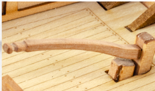
190. You can now glue the rudder into place. Slightly round/shape part #41 (as shown) and glue into place into the top of the rudder.
