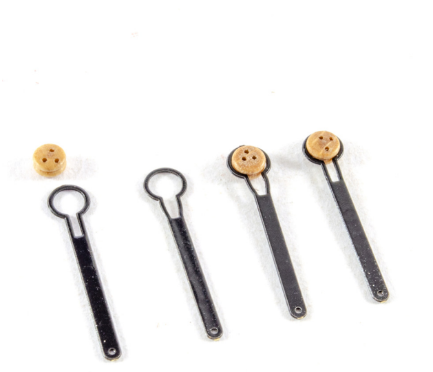
202. Take eight of the chainplates #PE-2 and paint them black. To fit the 3mm deadeyes to them, splay the part open as shown, place the deadeye into the loop, and then close up the area you splayed.
