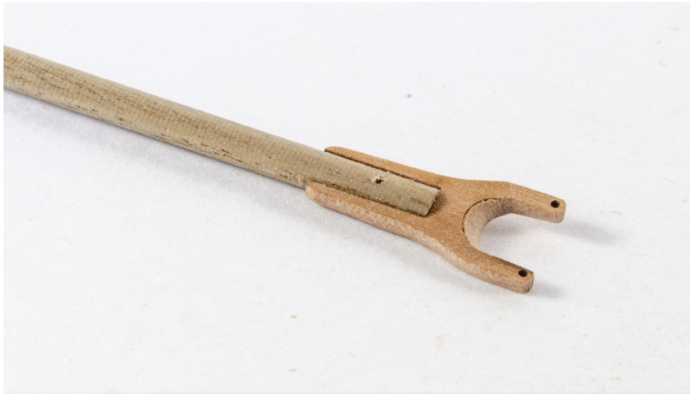
211. Here is a close up of main gaff, showing the jaws which have been bevelled up to the engraved line.
