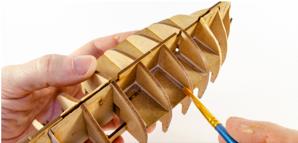
42. Paint slightly diluted wood glue into all the various joints and allow to fully dry. NOTE: There is nothing stopping the modeller gluing all parts as they build Saucy Jack, but due to the number of slots and type of construction, we generally advise applying the glue with a brush, after initial hull construction.
