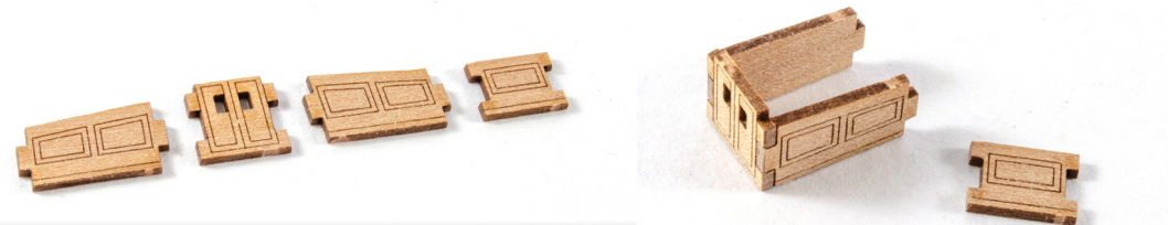
178. From the 1mm wood sheet, remove parts #60, #61, #62, and #63.
