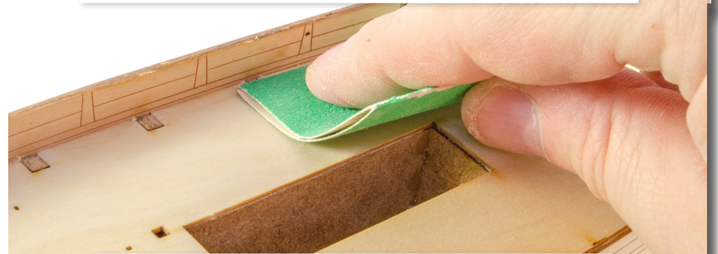
107. Use sandpaper to sand the stumps of the bulkhead ears flush to the deck.
