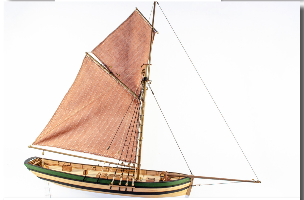
226. You can now rig the two mast sails as per your plan sheet. These aren't too difficult, and all the rigging lines are already attached. It's just like dot-to-dot.
