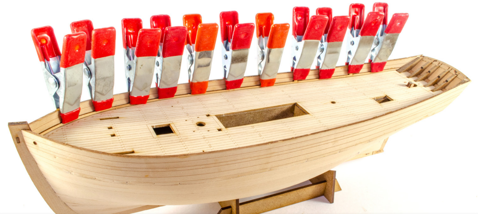
113. Fit the first #94 to the inner bulwark as shown. Clamp securely until dry. When dry, remove the clamps and repeat for the other side.
