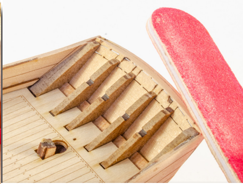
118. The stern is simply sanded flush along with the bulwarks. Just keep that sanding stick flat as you go over this area.
