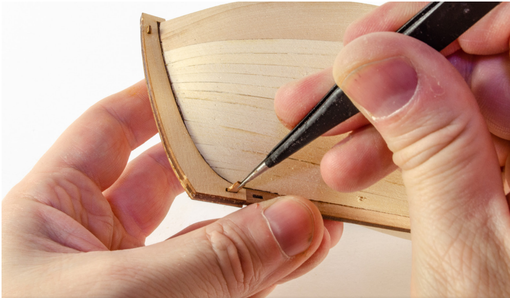
87. Glue the other part #82 to the opposite side of the hull and use the pegs #88 for alignment. Clamp until the glue is dry.
