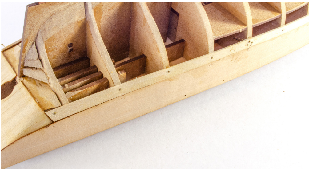
74. Here you can see the rear half of this plank run. You will need to glue the planks to each other, and to the bulkheads. Use the small brass pins to hold them in position while they dry.
