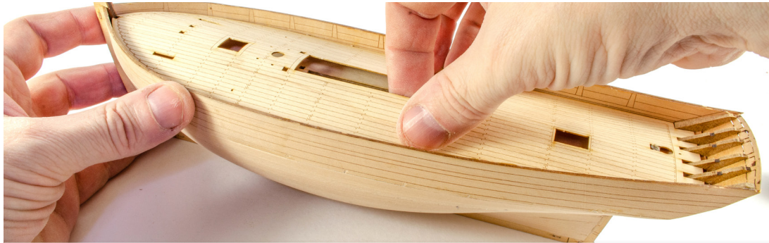
109. Test fit first by slightly bending the deck and ensuring it sits down on the ply deck, all the way around. If it doesn't, you may need to slightly sand the edge of the deck, where it's catching.
