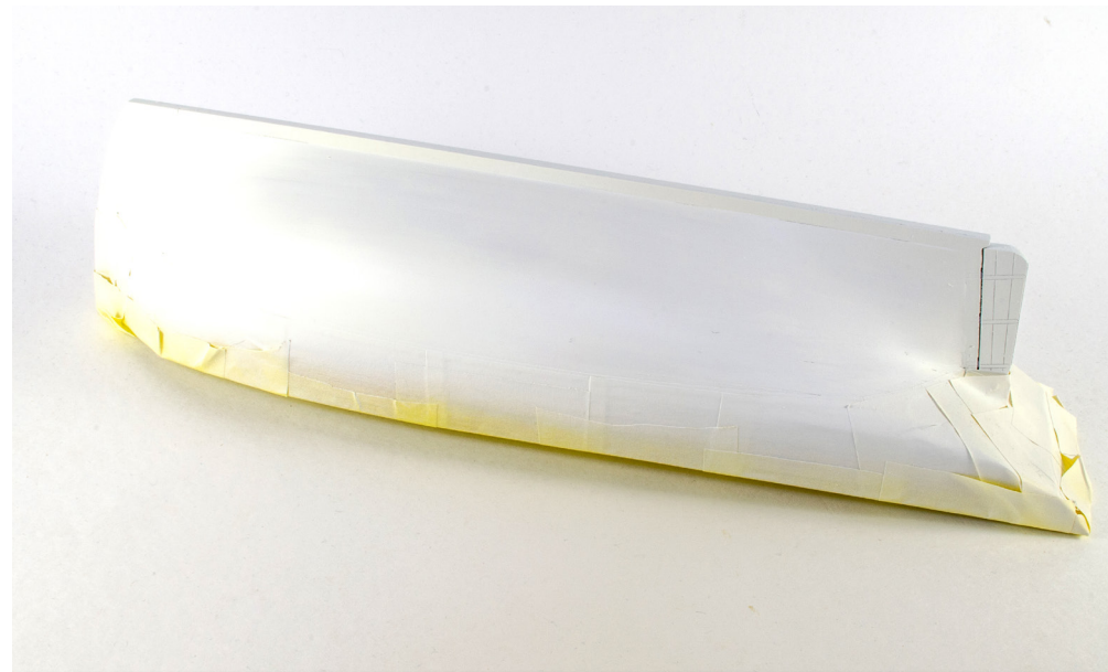
126. When you are happy with the primed surface, apply several thin coats of white paint. We use Plastikote White aerosol for this.
