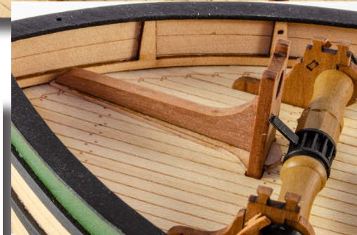
170. Glue into place. You need to bevel the long edge which sits against the previous assembly. You will also need to slightly angle the forward edge where it sits against the bulwark.
