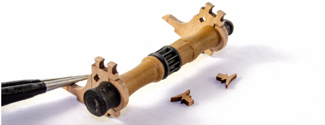
164. Paint the windlass drum in wood, with black for the metal areas. Trap this between the two wooden parts shown previously, making sure the engraved detail faces are pointing outwards. Also check this photo and your plan to make sure the windlass drum is the right way around. Try not to glue the wooden parts to the drum. You simply need to trap the part. From the 1mm wood sheet, remove both parts #70.
