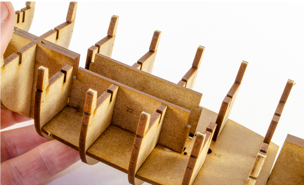
26. Glue both parts #22 into position on the deck. Getting these the right way round is easy as the part slots will only fit one way due to their length.
