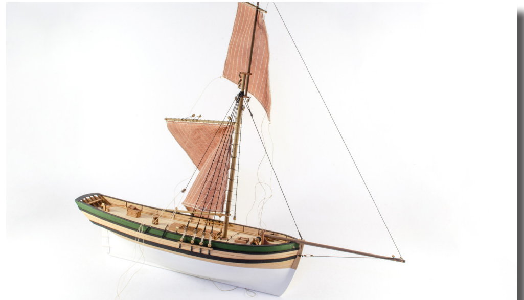
225. With the mast stays in place, add the two fore stays.
