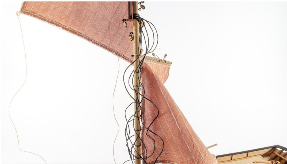
219. We now need to add the shrouds. These are lines which run from the mast step, down to the channels. Take a look at plan sheet #7 (standing rigging), for details on how these are applied. Leave the ends longer than is necessary.
