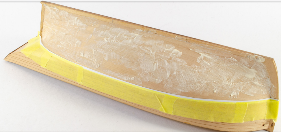
124. Mask the hull from the waterline, upwards, covering the bulwarks. We like to use flexible masking tape for the actual line, shown here in white. We also sell flexible masking tape in our webstore. Use wood filler to fill any imperfections or plank gaps on the exposed area. We suggest you use a good acrylic filler, diluted with water, and then applied with a brush.
