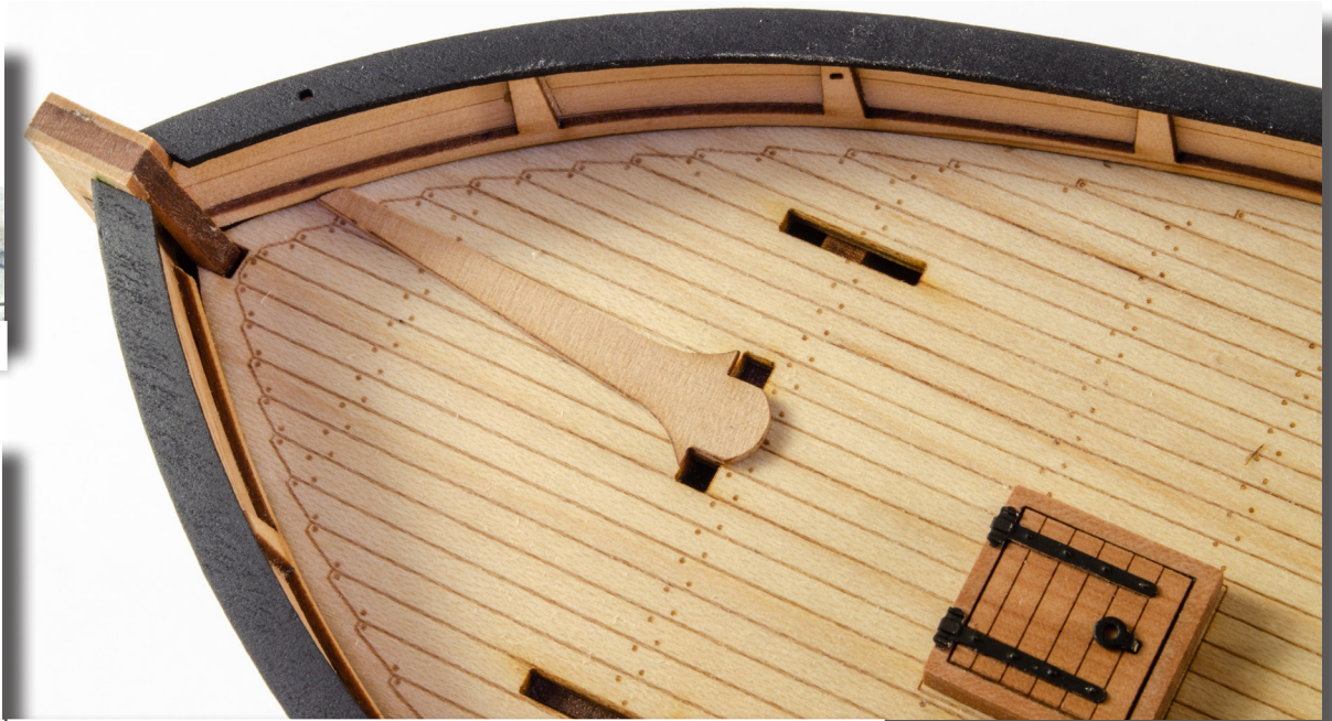
161. From the 0.8mm wood sheet, remove part #95 and glue into place as shown.
