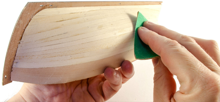
81. Use some sandpaper to sand the hull smooth. We suggest 110 grit paper to start, maybe finishing with something like 180 grit. That is up to you. Just don't sand it too thin. If necessary, you can use a little wood filler to remove any irregularities, and sand it in smooth to the shape of the hull.
