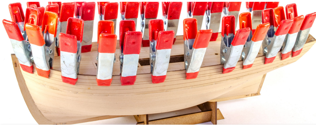
110. When happy with the fit, use slightly diluted wood glue to secure it. Use small clamps all the way around too, as this will ensure that it doesn't pop up anywhere.
