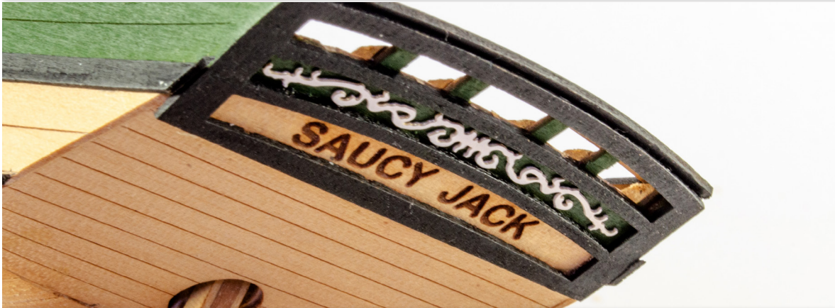
196. Paint the frieze part #21 and glue it into position in the blank stern panel. We chose white to give a nice but natural contrast.
