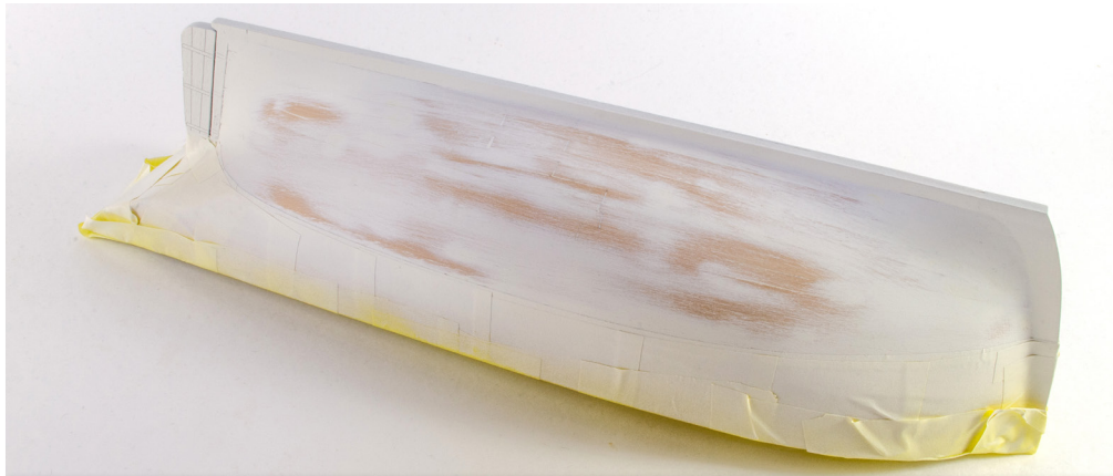
125. Apply a light coat or two of primer to the surface, and where you see an imperfection, simply refill and sand again. This can be tedious, but the result will be worth it.
