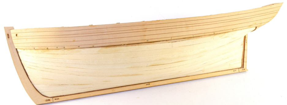
99. Take part #101 and glue into position as seen here. You will need to bevel the front edge a little, but the front area will now sit in the rebate that was created by the prow facings you recently added. This gives a good edge to plank up against. Clamp and use pins until the part is set. NOTE: You can use pins in the lower part of this outer bulwark as this will eventually be covered by the wales. When set, glue part #102 to the other side. You are now ready to add the second layer of pear planks.
