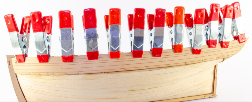
99. Take part #101 and glue into position as seen here. You will need to bevel the front edge a little, but the front area will now sit in the rebate that was created by the prow facings you recently added. This gives a good edge to plank up against. Clamp and use pins until the part is set. NOTE: You can use pins in the lower part of this outer bulwark as this will eventually be covered by the wales. When set, glue part #102 to the other side. You are now ready to add the second layer of pear planks.
