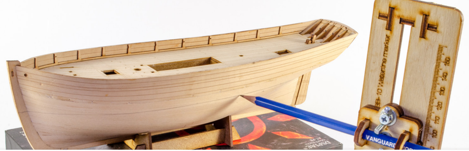
123. On your plan, measure the distance from the top of the wale (given here as the lowest engraved line on bulwark), down to the waterline, and then make a faint pencil mark. Check this distance from your plans. Now set your waterline tool to this mark, and draw a line from bow to stern, and over rudder, on both sides. NOTE: Before you do this, make sure that the bottom of keel is parallel to your worktop. This line will be parallel to your worktop and bottom edge of keel. Vanguard Models sell these waterline tools in the webstore.
