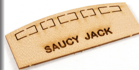
94. From the 0.8mm wood sheet, remove part #90. Note that we have kept the window blanks in place for the time being, as it aids strength.
