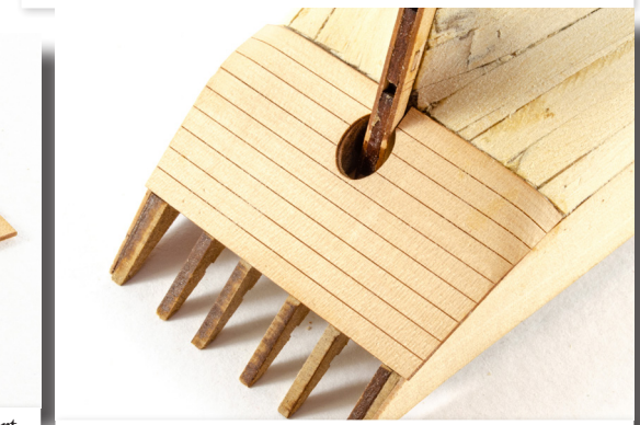
93. Soak this part for 30 minutes in hot water and then tape into place so the corners shape around the hull as shown. Leave this part to thoroughly dry for 24 hrs, then glue into position. It is necessary to leave the part to dry for so long because pear expands quite a lot until totally dry. NOTE: If you struggle to make the part bend around the corners, you can also use one of our plank nipping tools on our web store, and create nips in the underside corners, which will curl the part.
