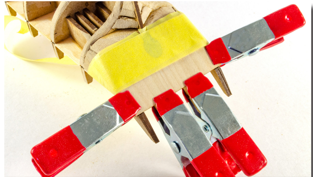
64. This part needs to be glued in place as shown here. The top edge of this will sit across the recess in the stern frames. Make sure this part has the rudder/post hole, central to the back edge of the keel. The part will overhand on both sides, equally. Use a combination of glue and clamps to hold in position until thoroughly set. The maple should wrap around the sides with no problems as it is very flexible.
